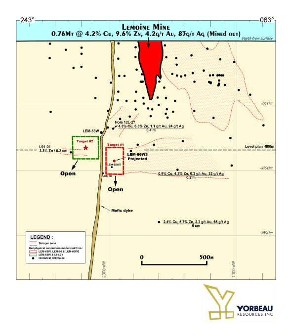
Figure 2 : Long section of Lemoine horizon, showing the revised modelled conductive plate of target #1.
