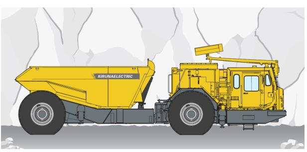
FIGURE 16-5 EM50T ELECTRIC MINE TRUCK
