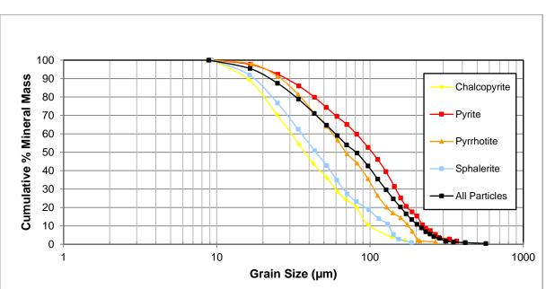
FIGURE 13-2 CUMULATIVE MINERAL MASS VS. GRAIN SIZE
