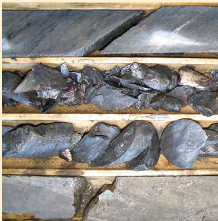
Hole 03-BES-3, 83.1m: Sulfides at the basalt-shale contact
