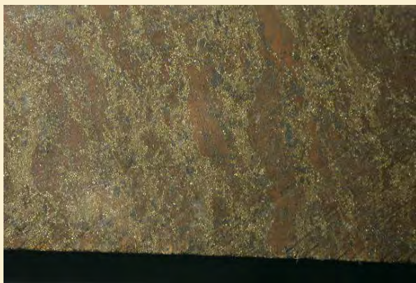
Hole 02-CBO-18, 310.9m: Heavily disseminated sulfides with Fe-carbonates
