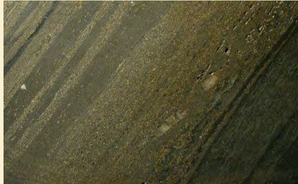
Hole 03-BES-04, 321.3 m: Semi-massive sulfides (pyrite, pyrrhotite with minor sphalerite and chalcopyrite)
