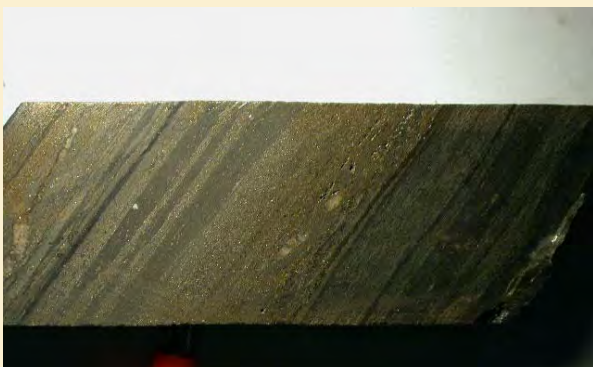
Hole 03-BES-04, 321.3 m: Semi-massive sulfides (pyrite, pyrrhotite with minor sphalerite and chalcopyrite)
