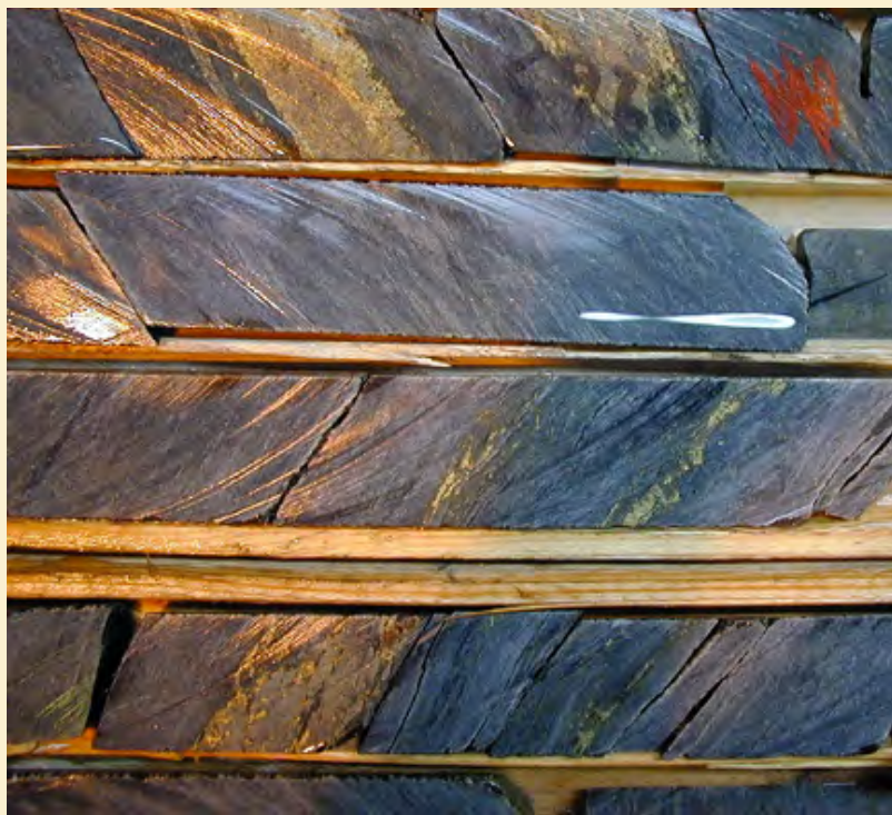
Hole 02-CBO-17, 1169.5m: Chalcopyrite – pyrrhotite veins from rhyolite A
