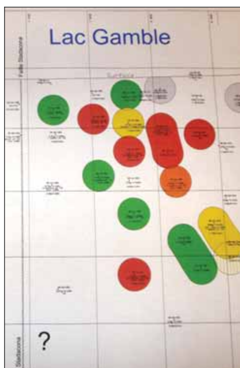
Figure 6 Yorbeau's drill intersections at Lac Gamble. Source: Yorbeau Resources Inc. [Red circles indicate intersections in excess of 25 g.m Au.]
